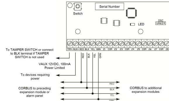
**TMP-** Used to tamper the cabinet in which the HSM2108 is mounted. Connect a normally closed (NC) switch across TAM and BLK. If the tamper is not being used connect a piece of wire across TMP and BLK to remove the trouble condition. There is a built-in tamper switch on the expander module located in the top left corner of the circuit board. If the cabinet in which the HSM2108 is mounted has the hardware required to depress this tamper switch, do not connect anything to the TAM terminal.
