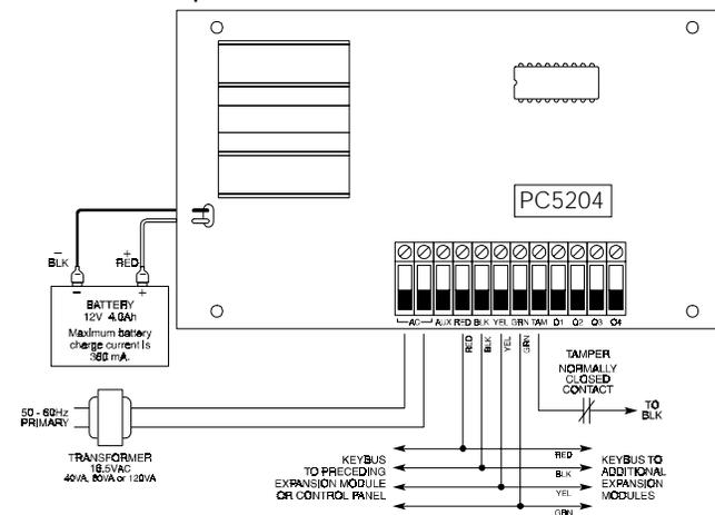
**AC** - The PC5204 requires a 16V, 40VA transformer. Connect the transformer to an unswitched AC source and connect the transformer to these terminals.
