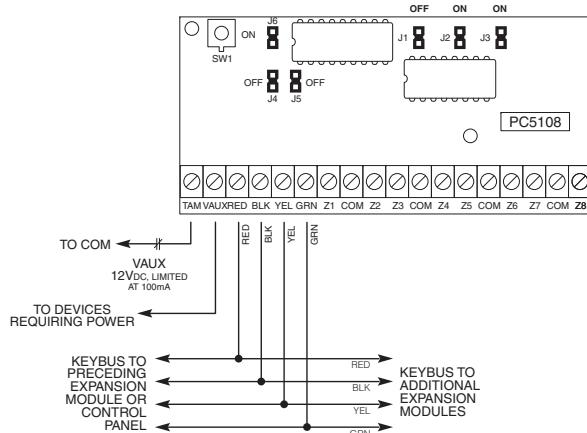
**TAM** - Used to tamper the cabinet in which the PC5108FLR is mounted. Connect a normally closed (NC) switch across TAM and BLK. If the tamper is not being used connect a piece of wire across TAM and BLK to remove the trouble condition.
