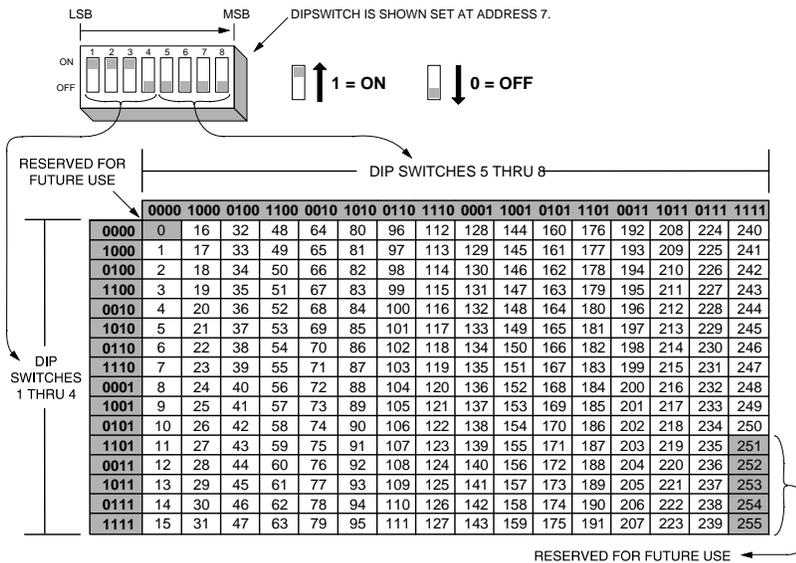
**Figure 2. Addressable IDNet Isolator Address Chart**
