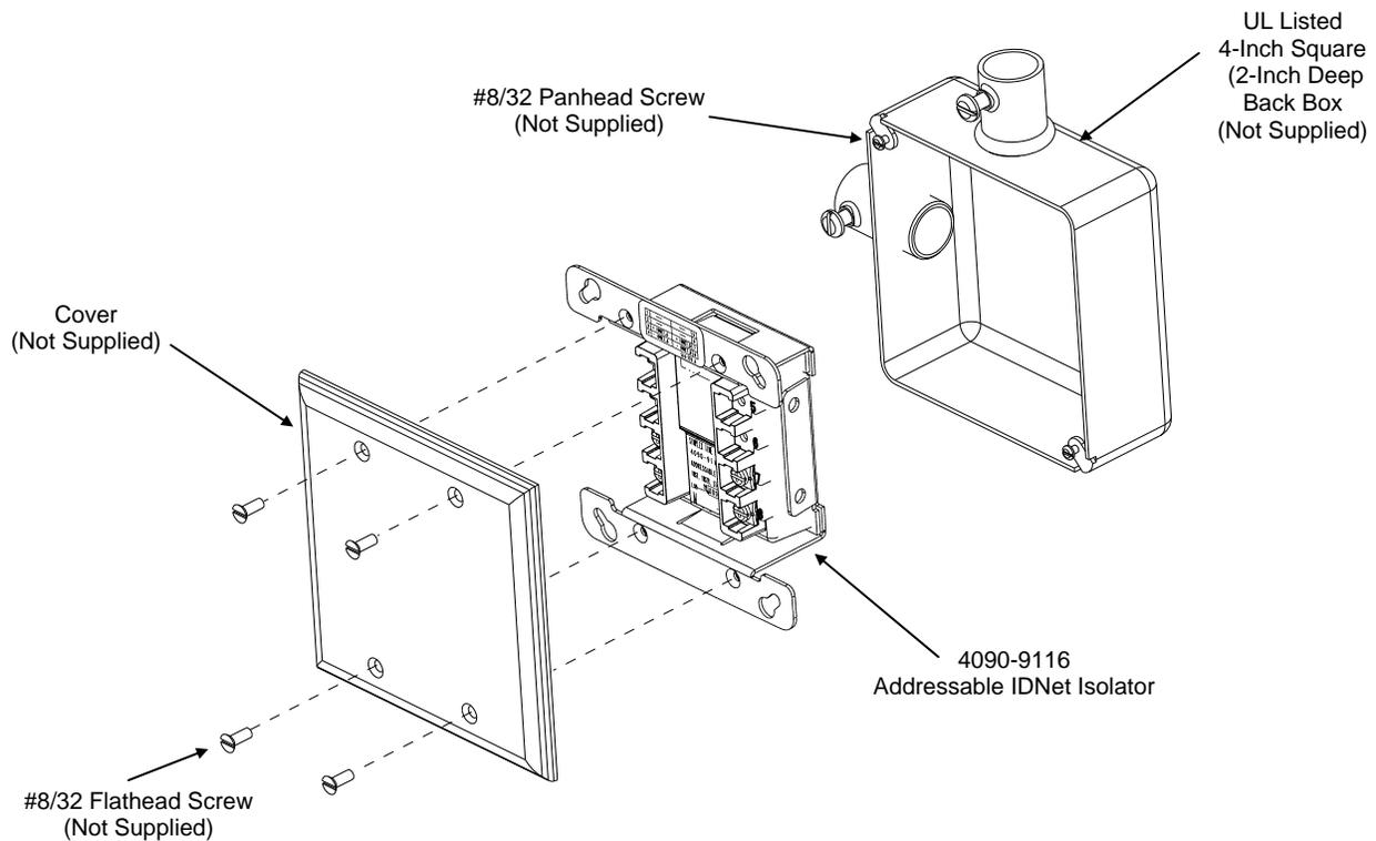
**Note:** Simplex offers semi-flush and surface covers (ordered separately) with a light pipe. The cover(s) with light pipe allow viewing of the communications LED without taking the cover off. Installation of the 4090-9806 semi-flush cover and 4090-9807 surface cover are detailed in publication *4090 IDNet™ Semi-Flush/Surface Covers and IAM Bracket Installation Instruction (574-796)*.
