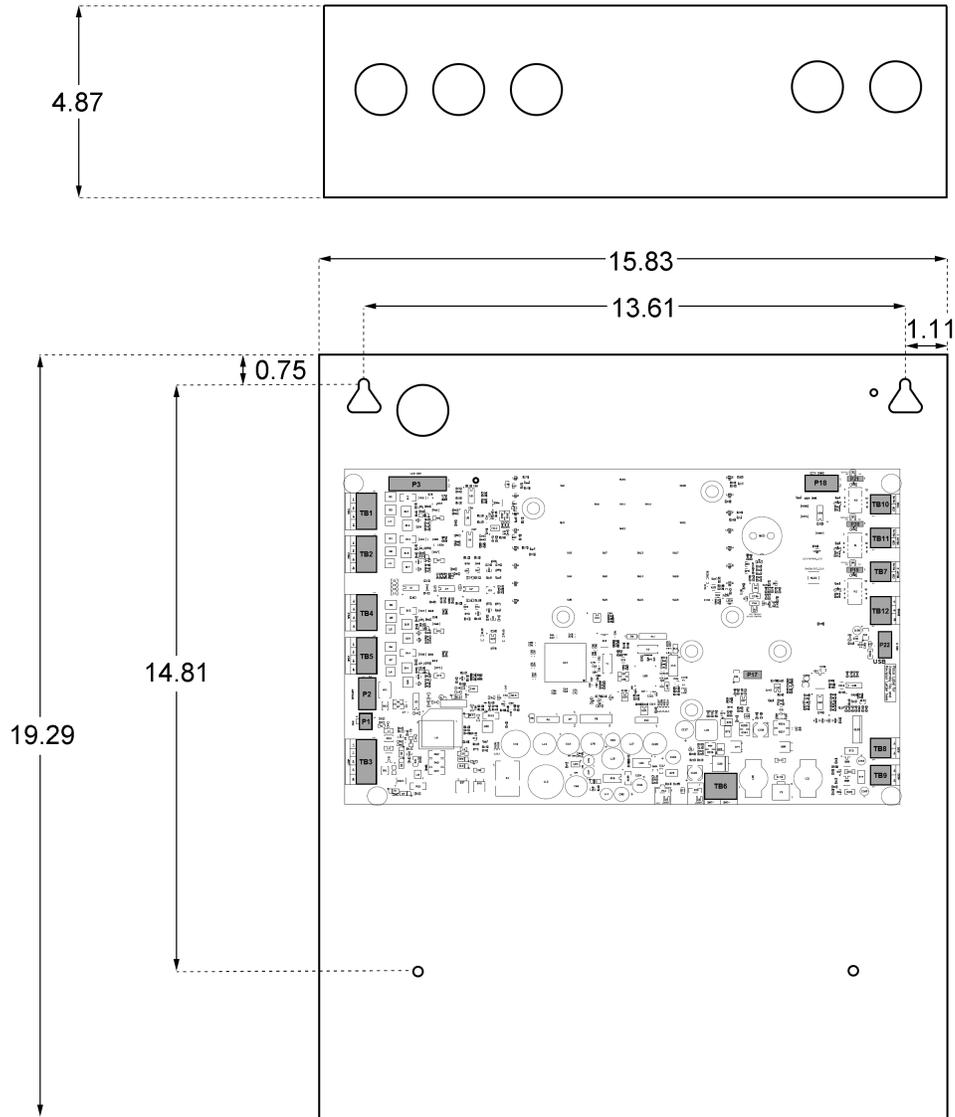
Figure 3: 2050FS control unit board
