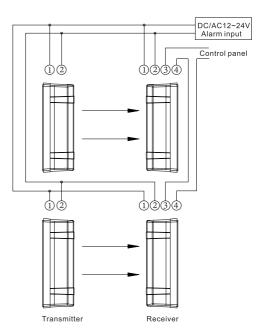
(3).2 pairs install in series: Connect power of transmitter and receiver in series with 12V DC on power supply. Alarm output is N.C.
