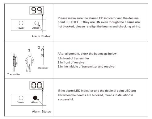
Note: If the alarm LED indicator is OFF even though the beams are completely blocked, refer to the "Trouble Shooting".
