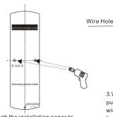
2. Attach the installation paper to the wall, mark the holes first and then make the guide holes.
