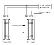
(2).Stacked connect: Control panel operating voltage DC12V,NC alarm output series connect
