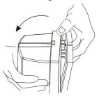
1. Loosen the screw and remove the cover
